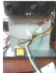
Remove the connectors from the cord and heater wires -
