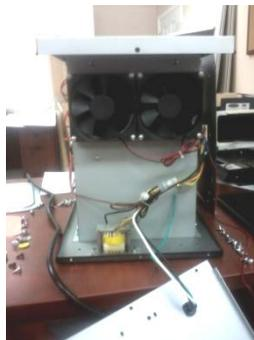
Next, connect up all the wires per the marks/photo and if at all possible solder the wires together before you screw on the new connectors. This will ensure a sound connection from the power cord to the heater wires. If solder is not an option, be sure to connect the wires very well before attaching the connectors, you need to have a good contact.
