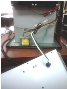
Remove the back metal panel from the top and sides and let it drop in front of you so that you can remove the wires as stated below.
