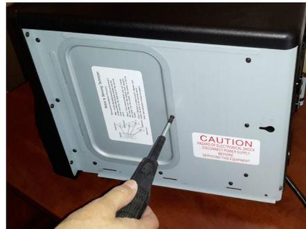
4. Remove the two screws to the fan switch or high-limit switch, depending on which switch is being replaced.
