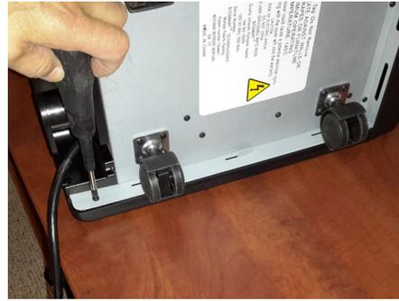
2. Slide the plastic side panel back 1/2 inch and pull out at the bottom. Remove the cover.
